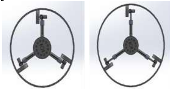
Fig.1 Robot in minimum and maximum pipe diameter
